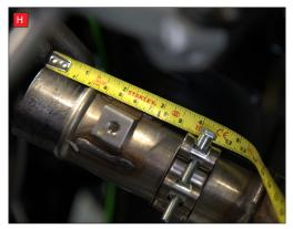
A) Loosen the clamp for the rear silencer.
