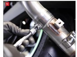
I) Place the plain clamp over the Scorpion connecting pipe then slide the pipe onto the original exhaust.
